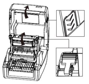
2.Pull the roll holders open and place the roll between them. And press down the locking tab.
