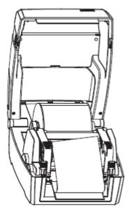
5. Wind the core 2~3 circles until the ribbon is pulled tightly.
