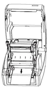
Note: If your printer is under Thermal Line Printing Method, press down the printer cover until it snaps closed. Otherwise, continue the procedure in chapter 3.1.2.
