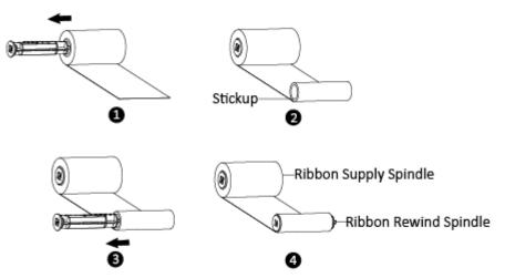
2. Insert the left part of supply spindle and then the right part.
